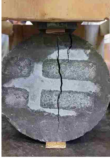
Figure 5-1 a) Front view of the Brazilian split cylinder
