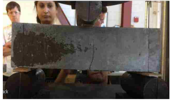
Figure b: Initiation of crack; back face
