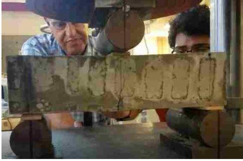
Figure a: Initiation of crack; front face
