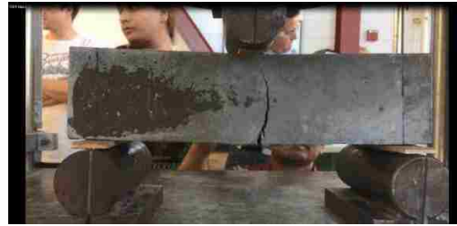
Figure d: Final crack; back face
