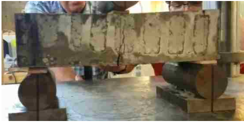
Figure c: Final crack; front face
